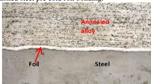
Fig. 1 Micro section of an annealed bimetal sample.
